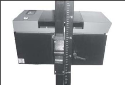
Position the optical box as shown in the photo. Attach with washer d.8 and M 8 x 20 screws, top left and with washer 8 x 24 (bigger) and snap lever M 8 x 20, bottom right.
