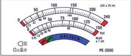
The analogical instrument has three scales, two of which are graduated and one of which is coloured.
